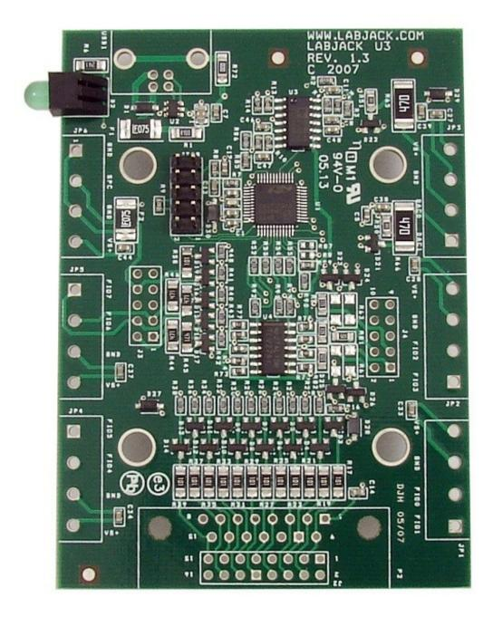
Screw-terminals are not installed. The PCB is designed for 5mm screw-terminals, but 5.08mm should fit also.
